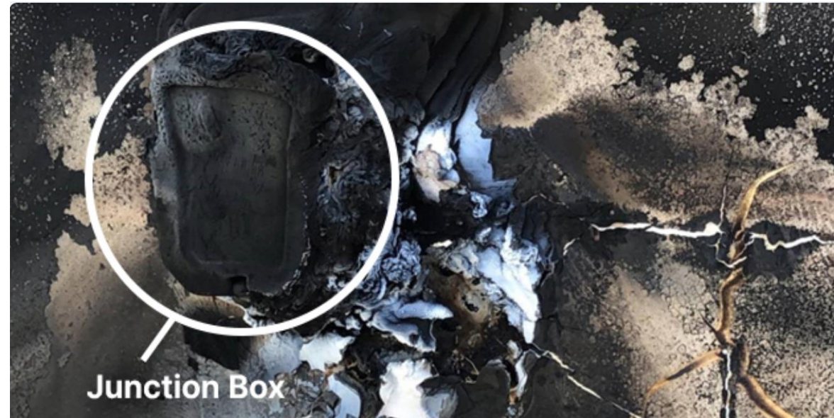
Image of extreme junction box failure 1
