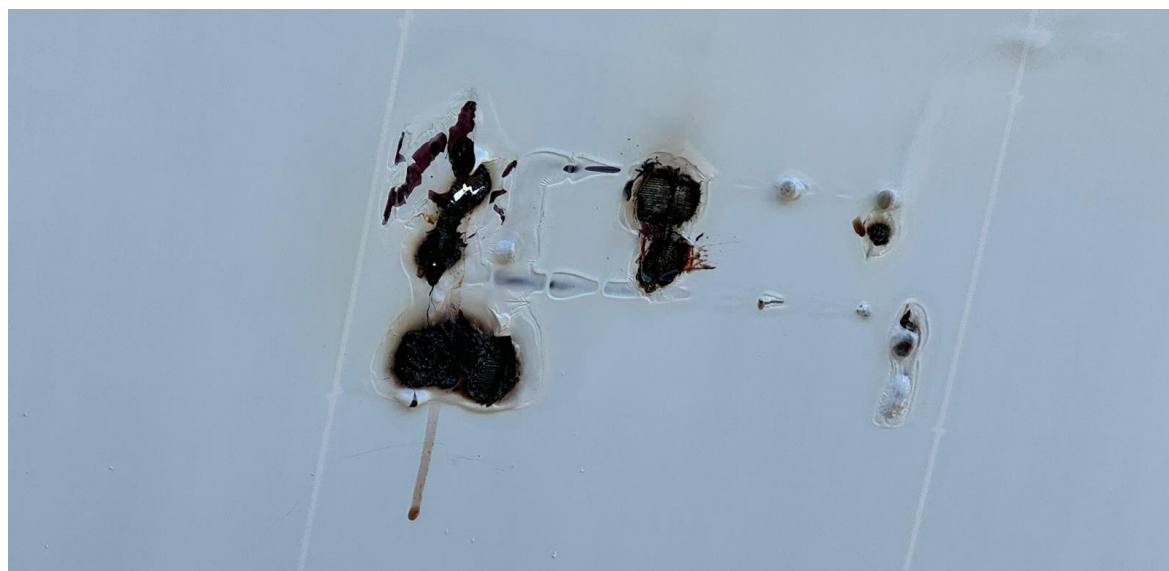
Fire damage following bypass diode failure
